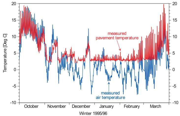
centric field of 91 bore-hole heat exchangers. In winter, heat is extracted from the heat storage and used to maintain a temperature of the bridge surface above 3 °C. SERSO provides a direct use of the geothermal heat. Electricity is only used for circulation pumps. The installation has shown that much more heat was collected in summer than needed in winter for de-icing. Experts agree that cooling in summer would also extend the lifetime of the pavement.
