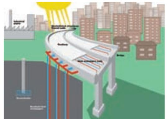
Geothermally heated outside surfaces are typically based on hydronic heat exchanger installations in the pavement. The installed heating capacity depends on the climatic conditions and the system specifications. Snow melting needs higher system temperatures than simple prevention of ice-formation. Low system temperatures implicate an anticipatory operation control.
