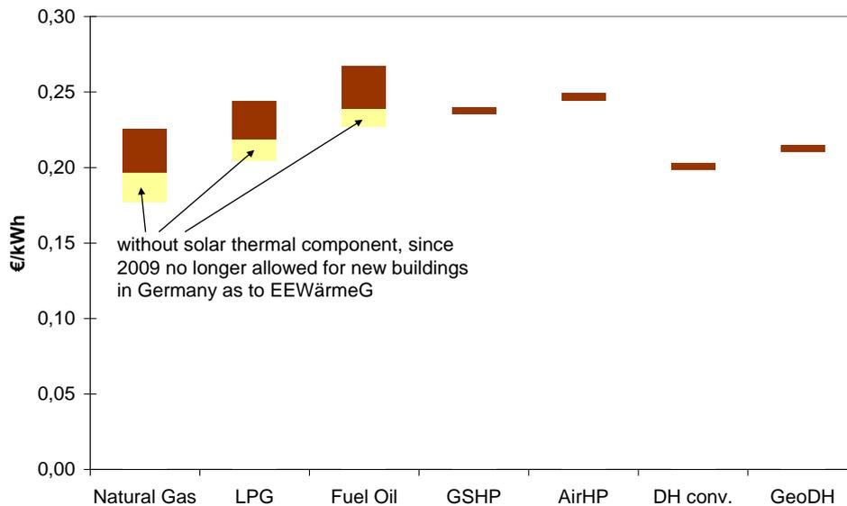
**Figure 5: Heat full cost in a modern residential house with 150 m<sup>2</sup> floor area in Germany in 2011, including all taxes and comprising the heat distribution in the building, after values from ASUE**
