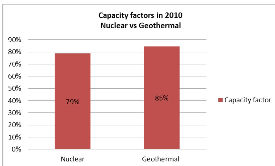
**Figure 1: Capacity factors in 2010: Nuclear vs Geothermal**
