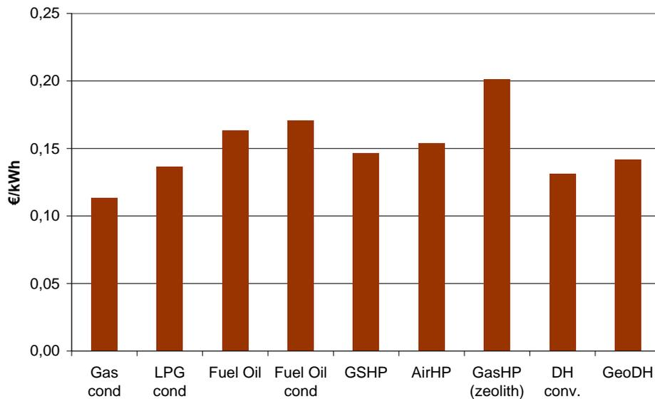
**Figure 6: Heat full cost in a modern residential house with 150 m<sup>2</sup> floor area in Germany in 2011, excluding VAT, solar components and heat distribution in the building, own calculation based upon values from ASUE**
